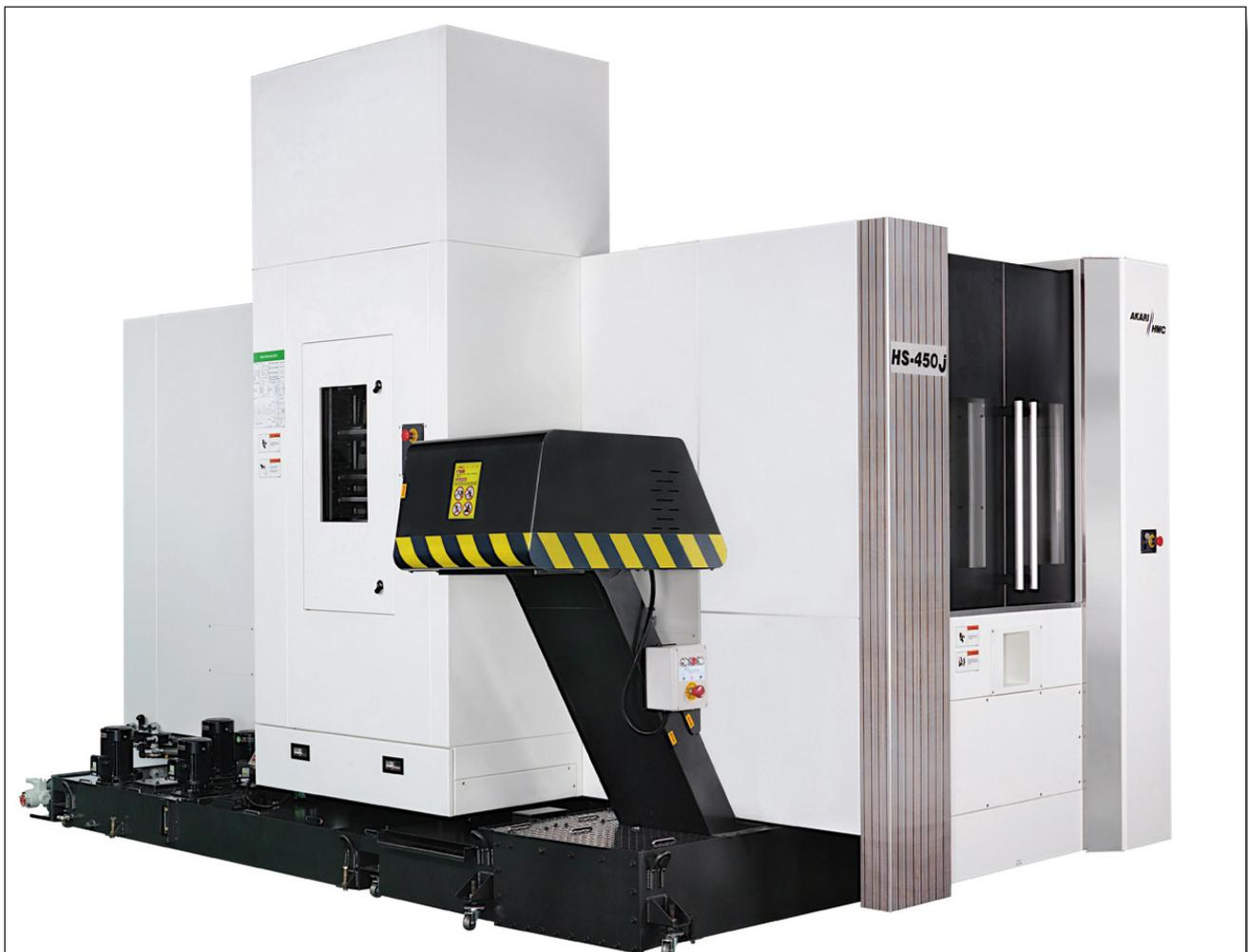
The one-piece bed casting, THK heavy duty roller guideways and BIG Plus 22 kW, 40-taper, direct drive spindle with 30 bar through-tool coolant remain the same. However, the standard full 4th axis rotary table has been replaced by a table with one degree indexing at 16.6 rpm, although the full (0.001 degree) 4th axis is available as an option.
