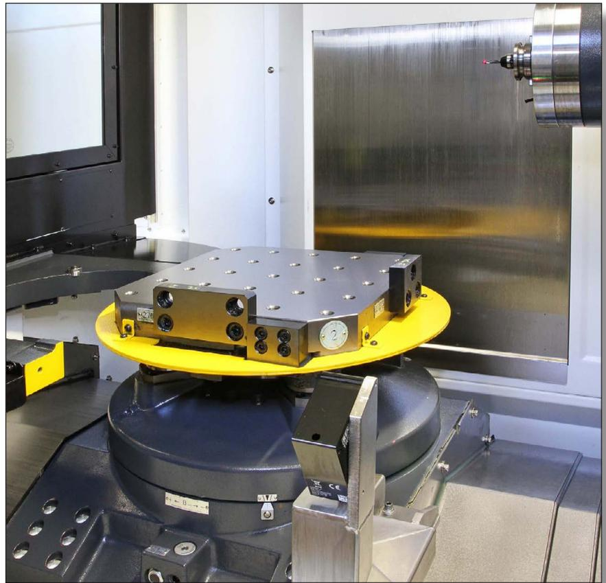
or 500 mm pallets are the maximum on the 450j and the choice of tool magazine is either 40 or 60 stations.
